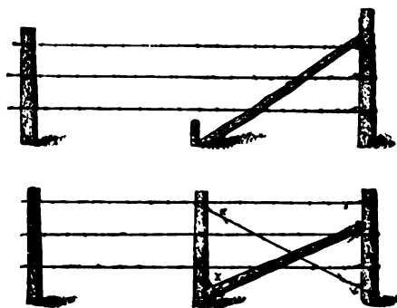
969. Illustrating the bracing of the end post in a fence or trellis.
